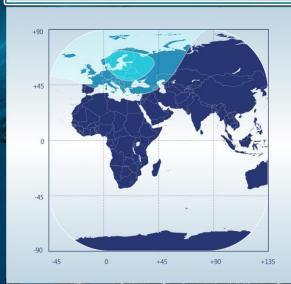
Ku-Band European beam Available bandw idth is: up to 4 x 54 MHz linear polarization Uplink: 12.75 – 13.0 GHz Dow nlink: 10.7 – 10.95 GHz
