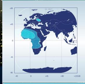
Ku-Band African beam Available bandw idth is: up to 12 x 36 MHz linear polarization Uplink: 14.00 – 14.50 GHz Dow nlink: 10.95 – 11.20 GHz 11.45 – 11.70 GHz
