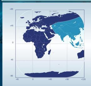
C-Band, Eastern beam Available bandw idth is: up to 8\* x 36 MHz circular polarization Uplink: 5 725 - 6 725 MHz Dow nlink: 3 400 – 4 200 MHz
