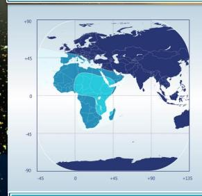
C-Band, African beam Available bandw idth is: up to (8+8\*) x 36 MHz circular polarization Uplink: 5 725 – 6 725 MHz Dow nlink: 3 400 – 4 200 MHz
